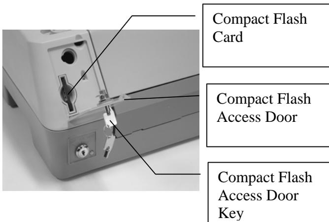
22. Using the Access Door key provided, unlock the Access Door containing the compact flash card.
