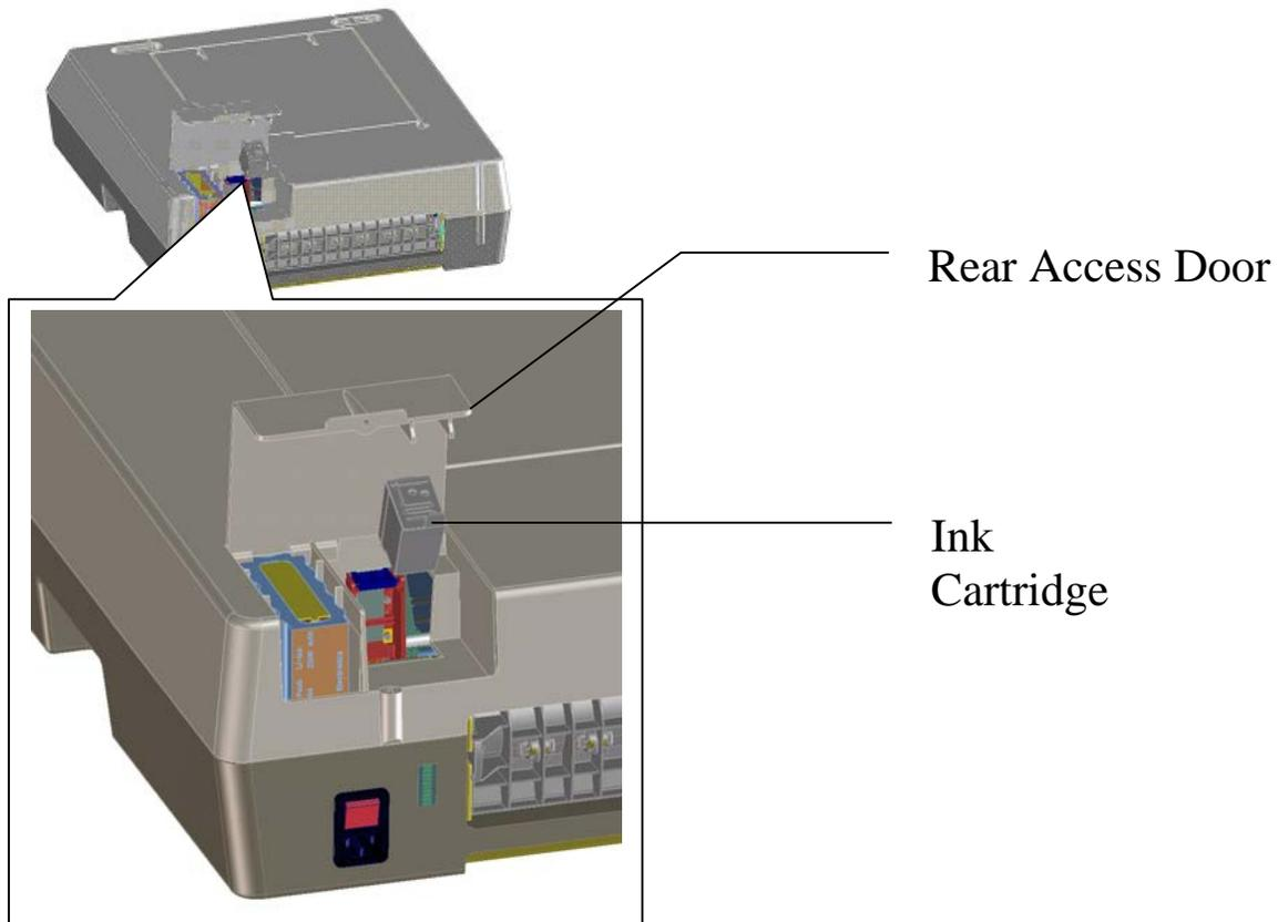
25. Remove the screw or snap that secures the Rear Access Door. Open the Door.
