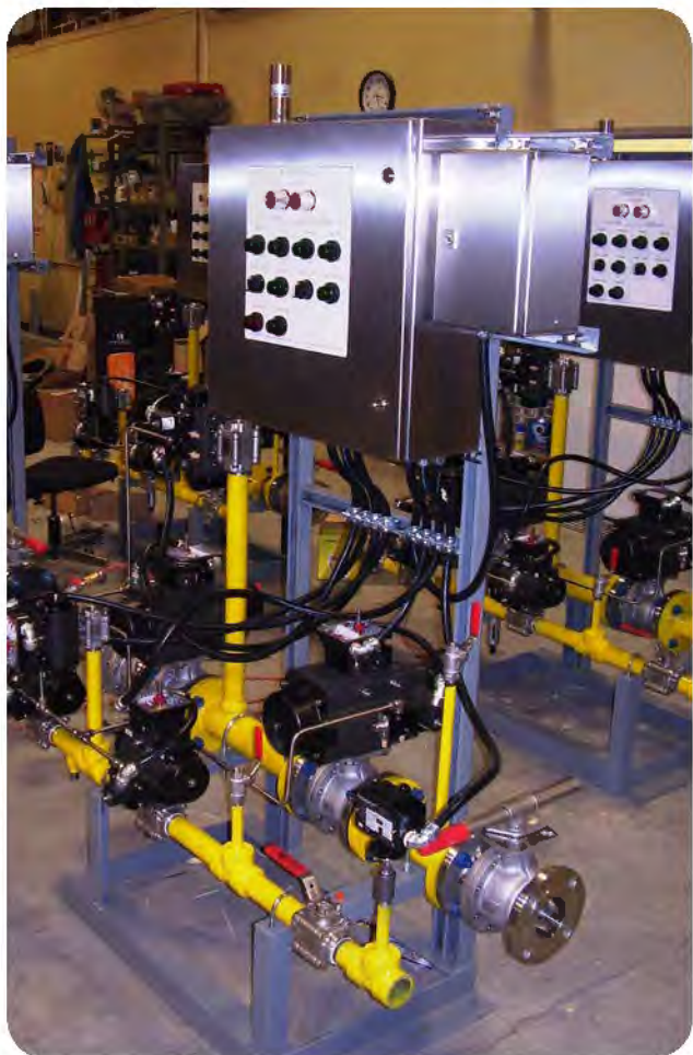
Burner/igniter valve train with local control panel.
