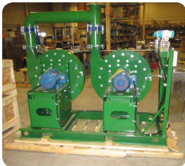
Duplex cooling air blower assembly.
