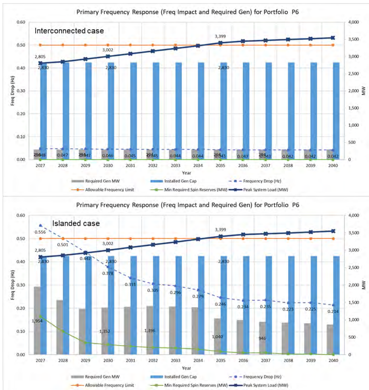
Figure 60. Primary frequency response for Interconnected and Islanded case for portfolio P6
