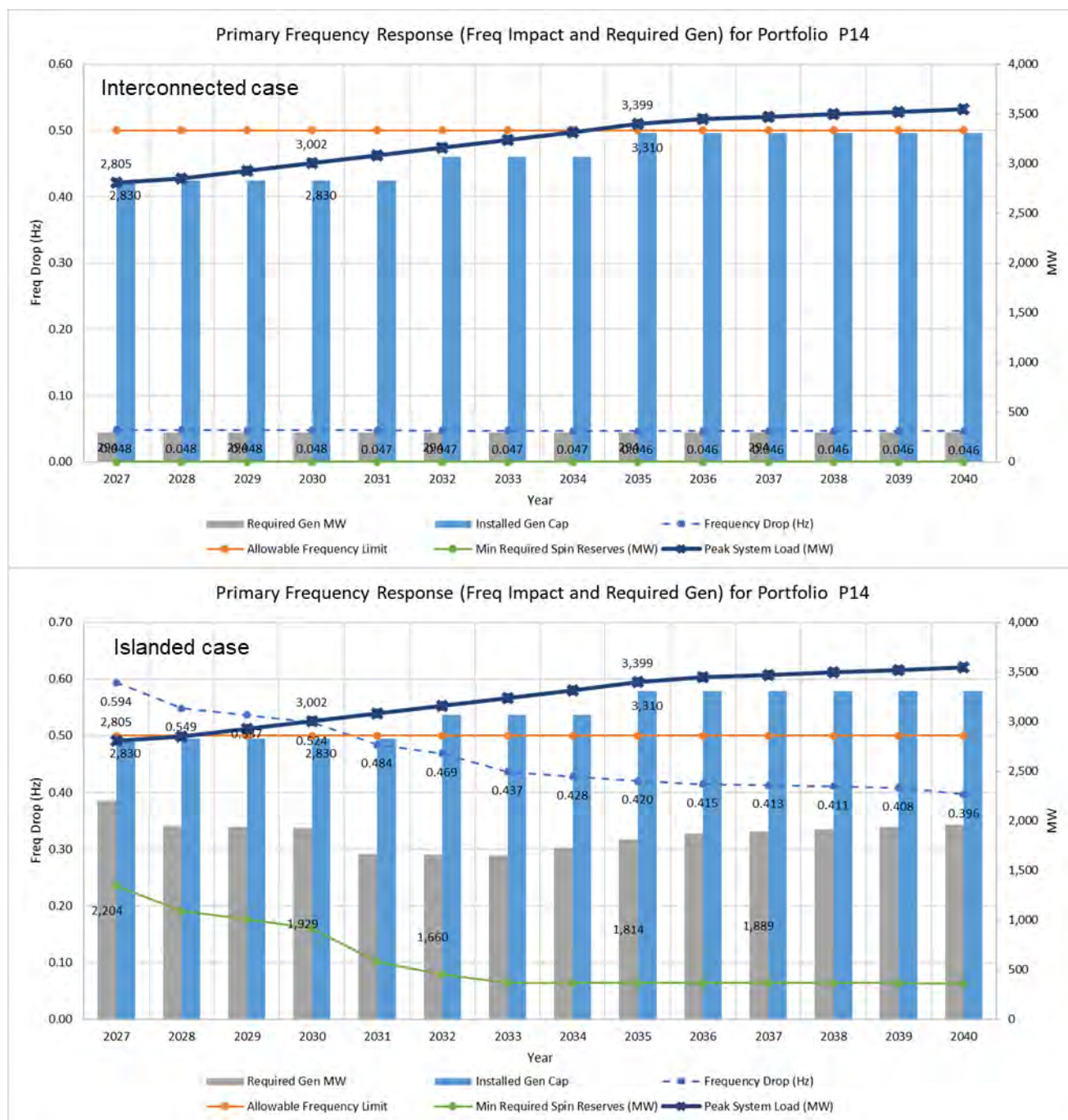
Figure 68. Primary frequency response for Interconnected and Islanded case for portfolio P14
