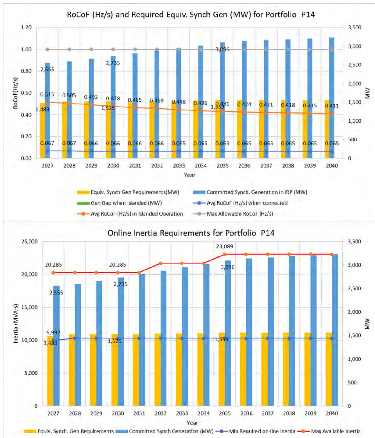
Figure 52. Synchronous Generation Requirements and Expected RoCoF and Online Inertia Requirements for Portfolio 14
