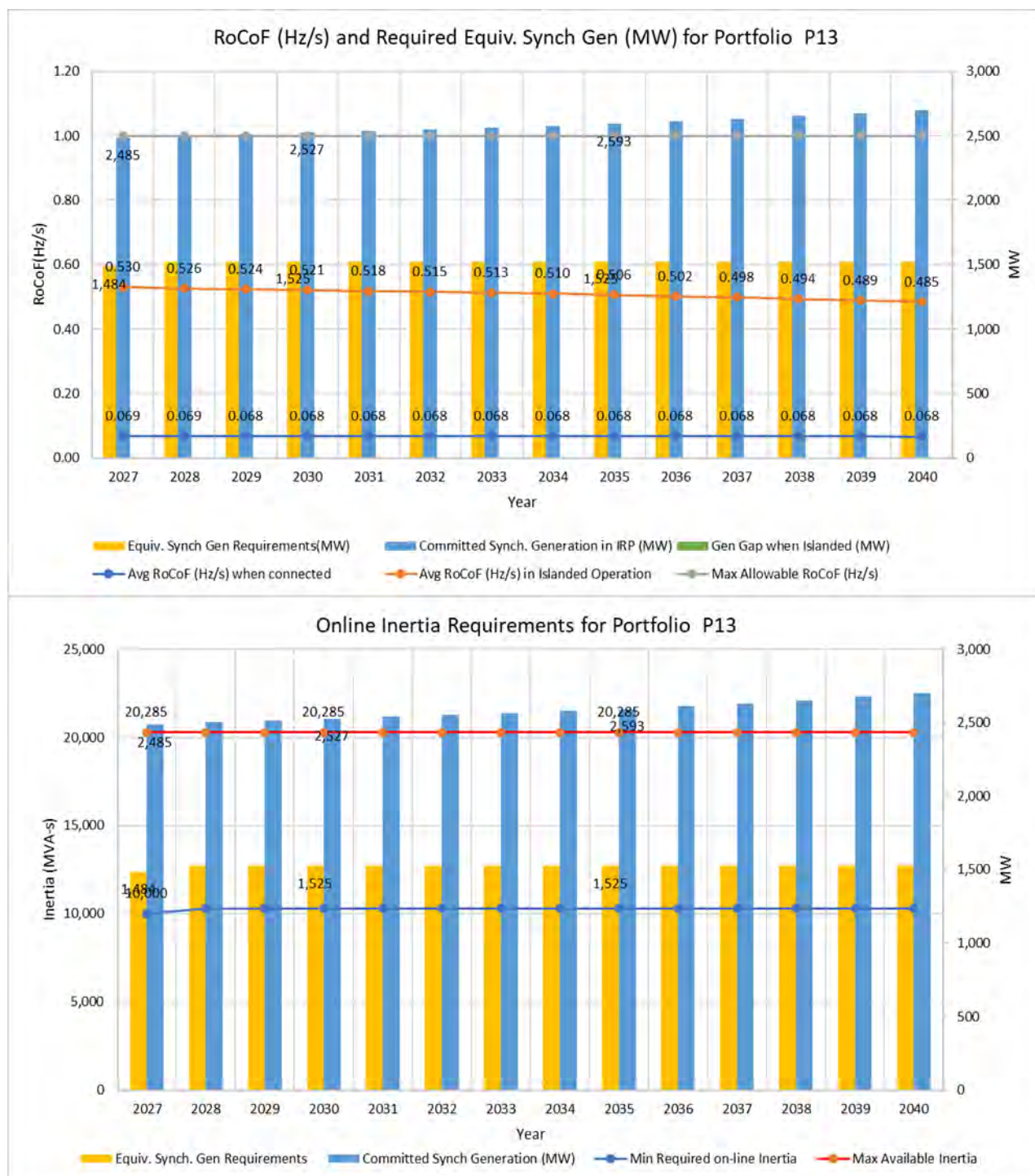
Figure 51. Synchronous Generation Requirements and Expected RoCoF and Online Inertia Requirements for Portfolio 13
