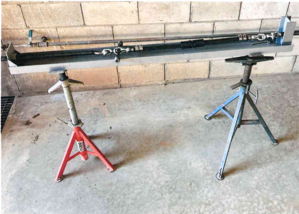
Mechanical Coupling Testing Apparatus with 3/4" PE and Lycofit to be tested
