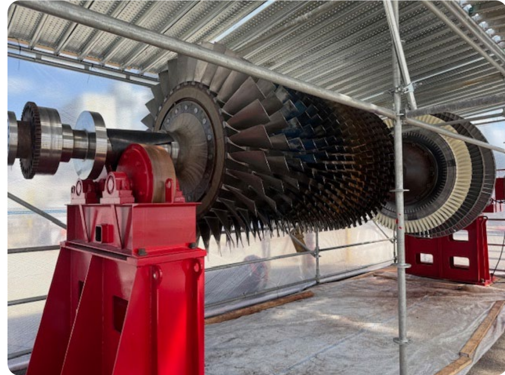
Madison Combustion Turbine Unit 5 Rotor
