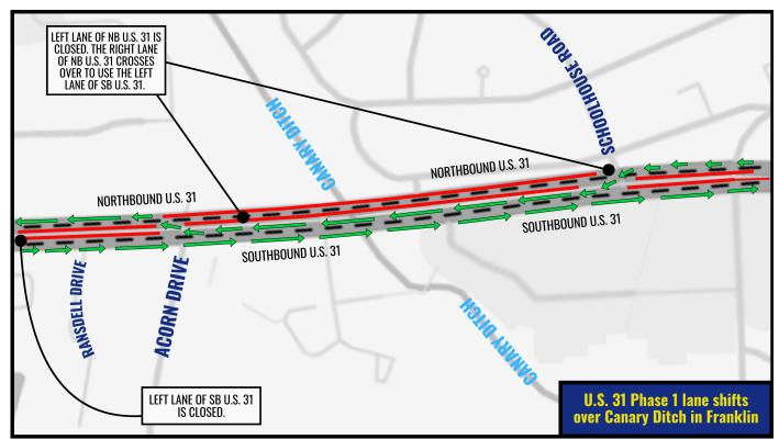
(Map display: U.S. 31 Phase 1 lane shifts over Canary Ditch for box culvert replacement in Franklin. Not to scale.)
