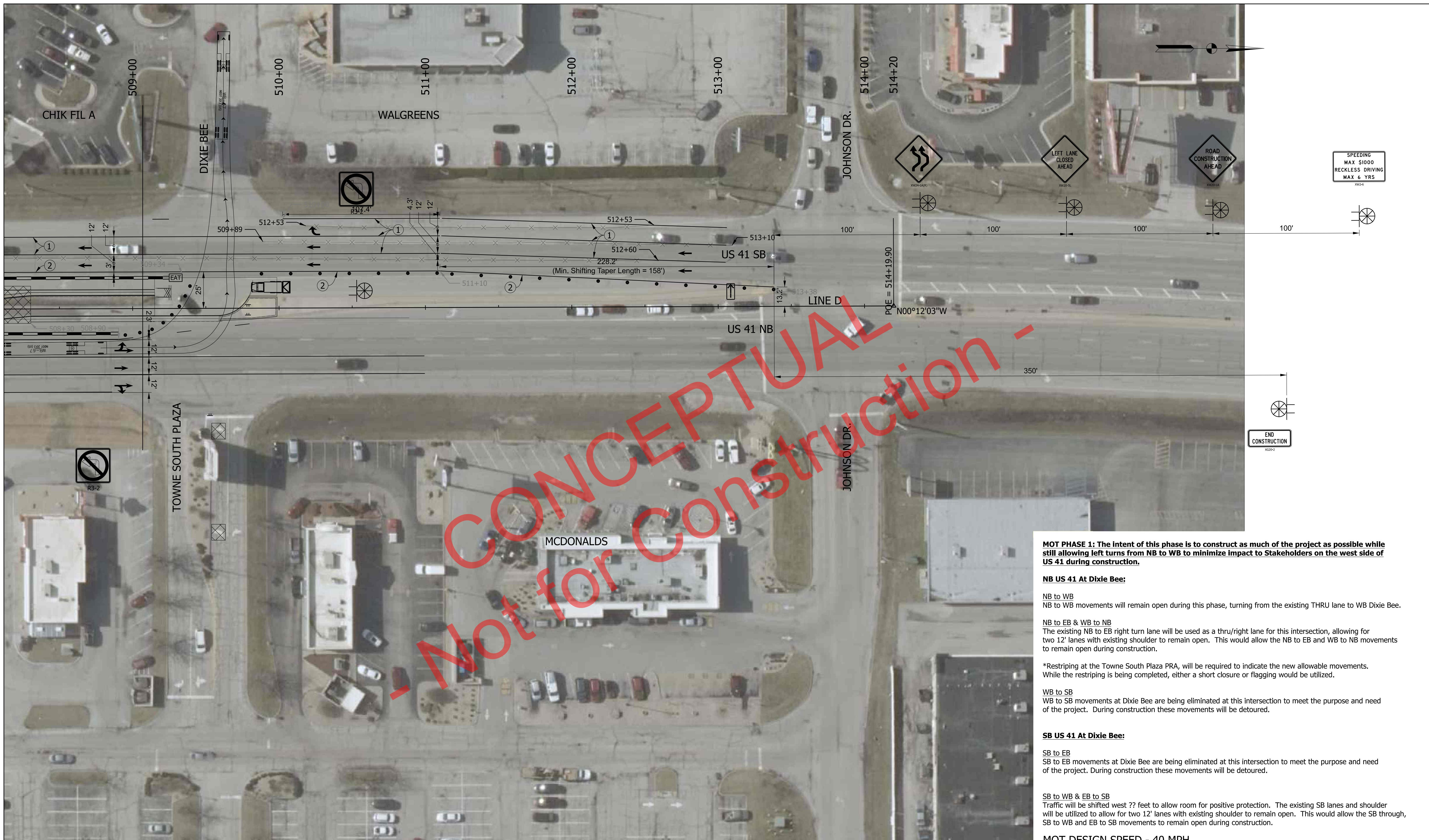
**MOT PHASE 1:** The intent of this phase is to construct as much of the project as possible while still allowing left turns from NB to WB to minimize impact to Stakeholders on the west side of US 41 during construction.
