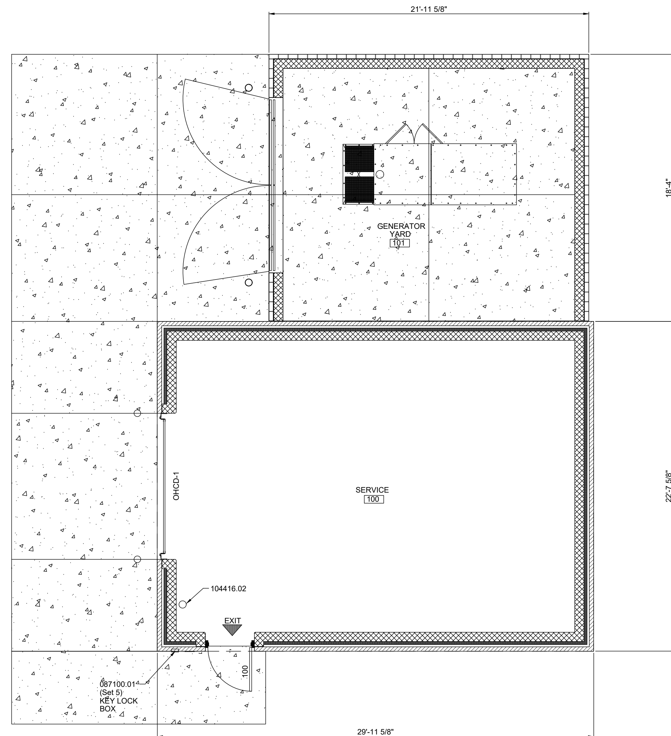
MAINTENANCE BUILDING LIFE SAFETY PLAN
