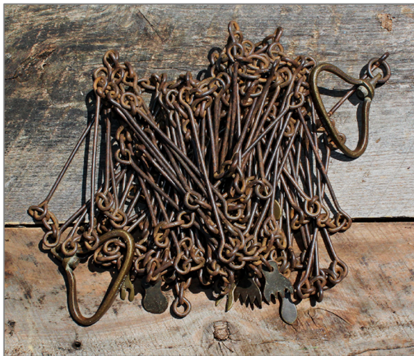
Figure 7.7-1: Gunter’s Chain used in early U.S. Public Land Surveys.
