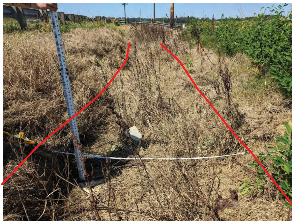
Photograph 46. The downstream view of the OHWM taken for UNT to Willow Pond Ditch, which contains minor intermittent vegetation below scour marks, looking west.
