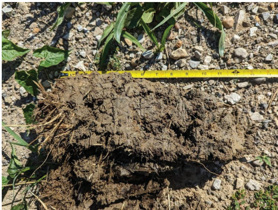
Photograph 6. View of the soil profile of SP1 within Wetland A, which met the A2, A3, C2, C3, D2, and D5 wetland hydrology indicators. Saturation was observed at 7 inches.
