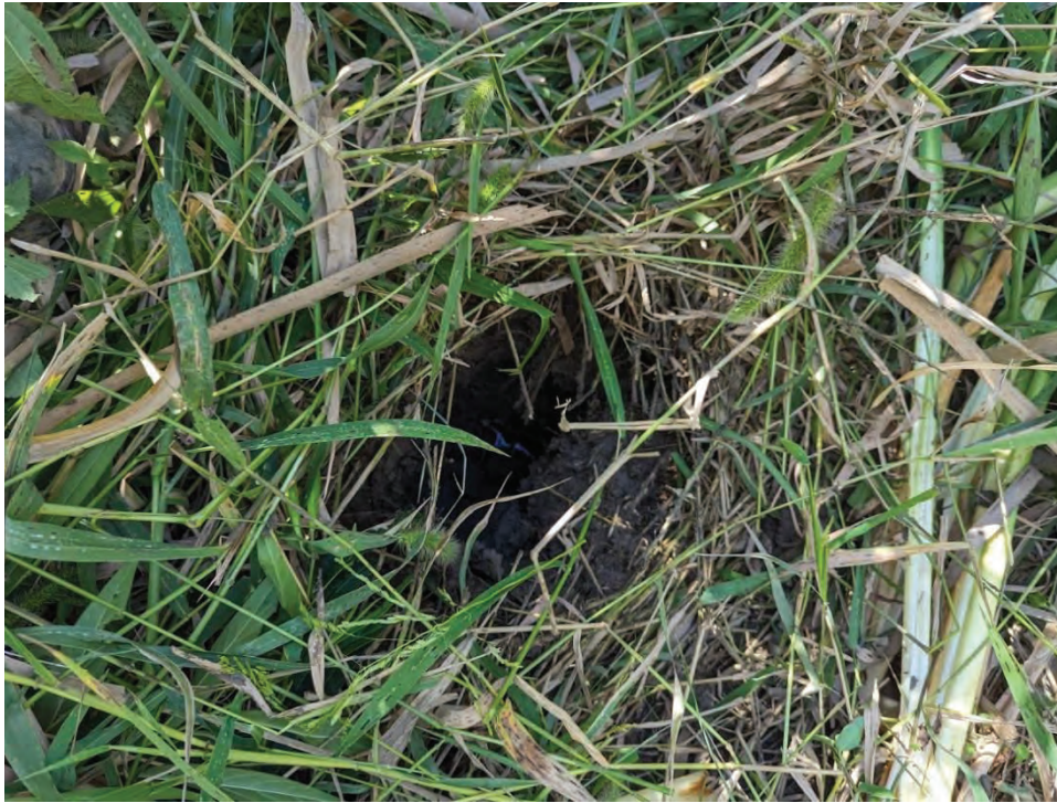
Photograph 7. View of the soil pit of SP1 within Wetland A where a high water table was found at 12 inches.
