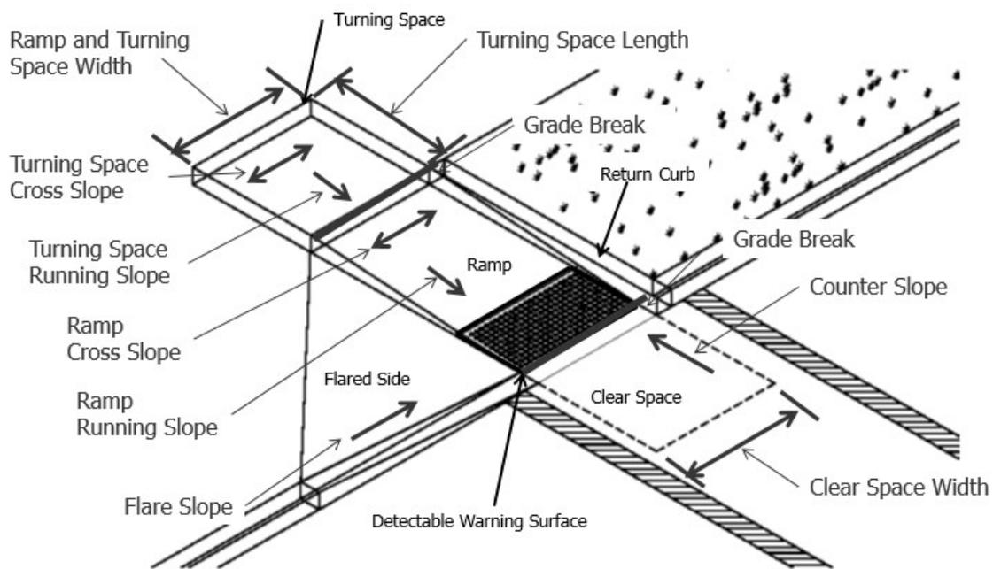
Turning Space must be level with both running and cross slopes < 2%, meaning these slopes should be designed at < 1.5% to ensure a compliant result.
