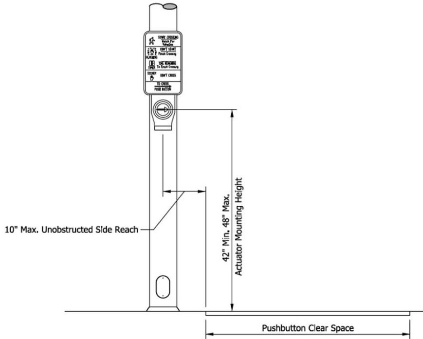
The Pushbutton clear space should be a 4' x 4' level area where the running and cross slopes do not exceed 2%. Slopes of all level areas should be designed to <1.5% to ensure a compliant result. If the signal is not an APS signal, it must still have a 2" button and comply with all button reach and mounting height requirements.
