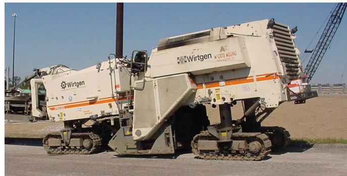
Figure 7-3 Deck Surface Milling/Scarifying Machine
