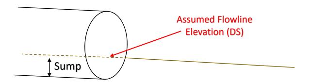
Assumed flowline is the elevation of the flowline above the outlet invert.
