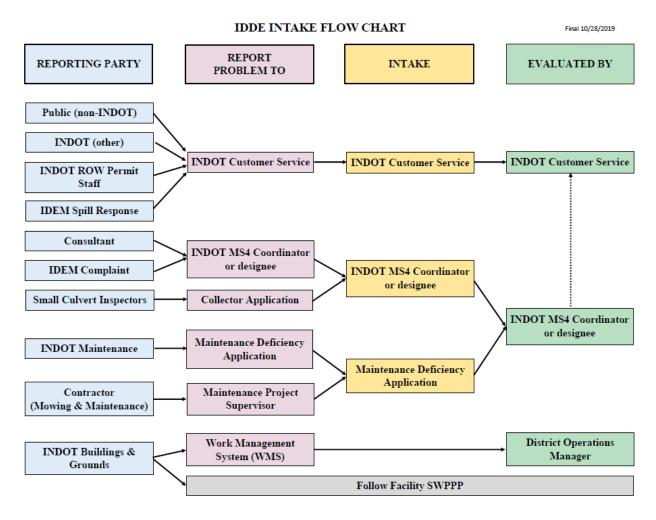
The IDDE Problem Evaluation flow chart was developed as part of the IDDE plan. It provides a process for evaluating problems based on the location and type. It provides the lead for investigation and resolution and a reporting path.
