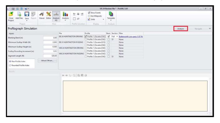
12) Once the analysis is complete, the profilograph simulation results will be available as a chart and in table form as shown below. There are scrolls both vertical and horizontal to allow viewing of the results. Next, select **Navigate** in the upper right corner and click on **Scallops** for the remaining portion of the analysis.
