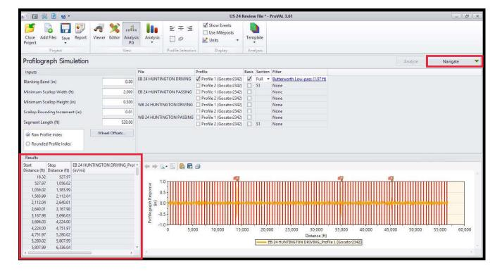
13) Once the 2<sup>nd</sup> portion of the analysis is complete, the profilograph scallop results will be available as a chart and in table form as shown below. There is a scroll to allow viewing of the results which will indicate each location where the 0.3 inch deviation threshold was exceeded.
