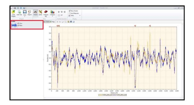
5) Next, the section needs to be identified for analysis. Not all sections start at 0 feet as can be seen above in the example. The starting feet on this graph needs to correspond with a station that represents the start of paving. To identify the section, select the **Editor** icon. Now select which file you want to use from the File dropdown.
