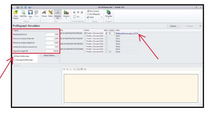
11) Now that the Profilograph Simulation has been set to meet the specifications, and the file to be analyzed has been selected and filtering is set. Click the **Analyze** button in the top right corner.
