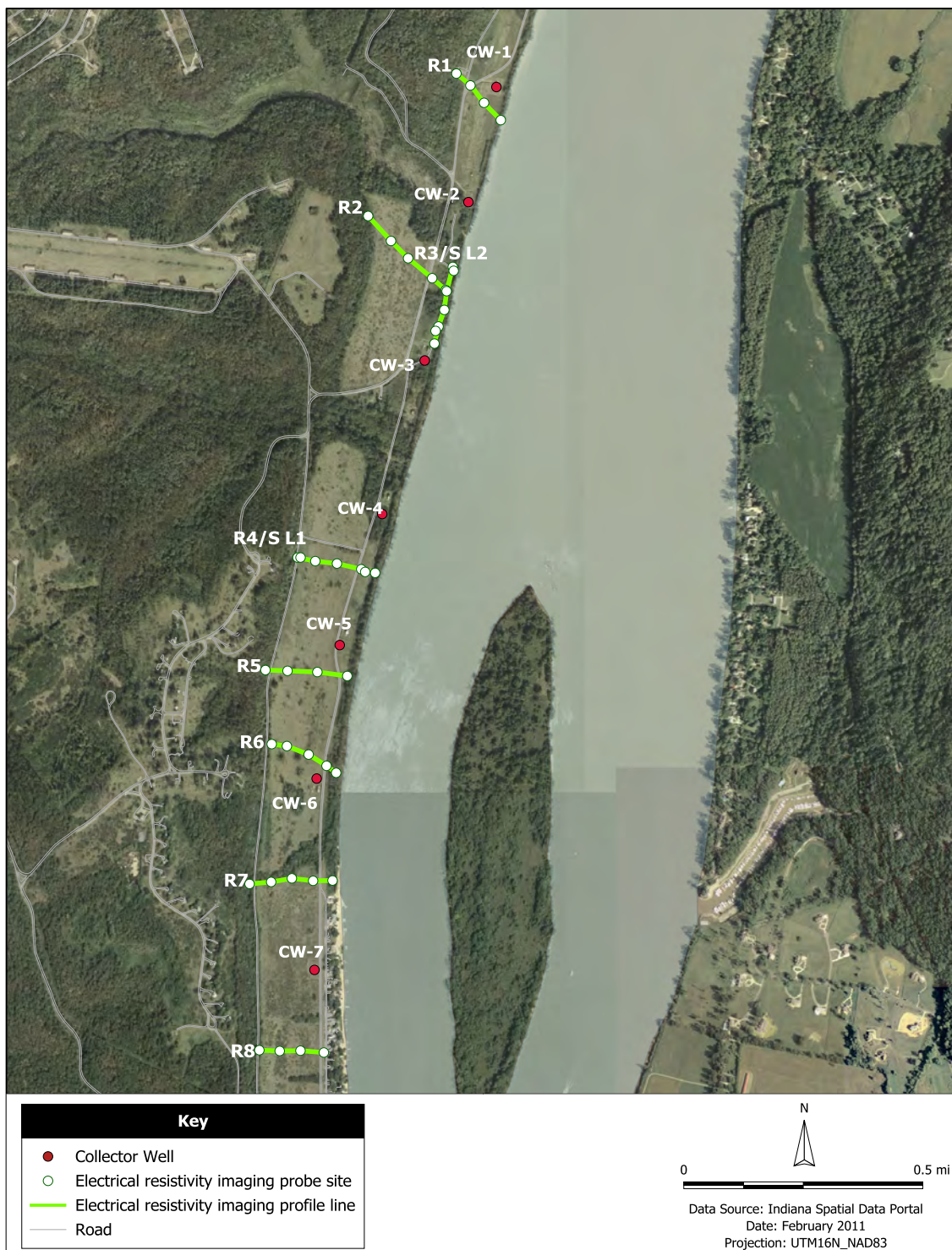
Figure 4: Location of the land electrical resistivity profiles R1 through R8 and seismic lines SL1 and SL2.
