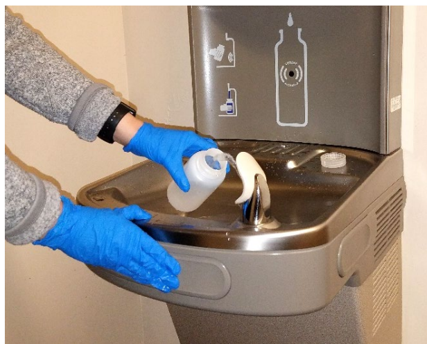
Figure 6. A Technical Assistance Provider (TAP) sampling drinking water from a drinking water cooler . A water cooler is a fixture that dispenses chilled water. This is in contrast to a drinking water fountain that dispenses room-temperature water if installed indoors, and ambient temperature water if installed outdoors.
