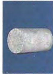
Louisville Tunnel Project 1831-10-5629 South Bound Boring 2 (Run 46 Box 33) 416.7' (Unconfined)
