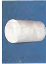
Louisville Tunnel Project 1831-10-5629 South Bound Boring 12 (Run 107 Box 73) 1,004.3' (Unconfined)
