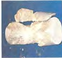
Louisville Tunnel Project 1831-10-5629 South Bound Boring 9 (Run 88 Box 60) 824.7' (Unconfined)
