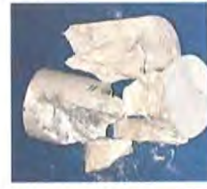
Louisville Tunnel Project 1831-10-5629 South Bound Boring 11 (Run 100 Box 69) 942.9' (Unconfined)
