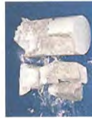
Louisville Tunnel Project 1831-10-5629 South Bound Boring 12 (Run 107 Box 73) 1,004.3' (Unconfined)
