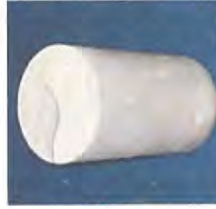
Louisville Tunnel Project 1831-10-5629 South Bound Boring 13 (Run 113 Box 77) 1,064.2' (Unconfined)
