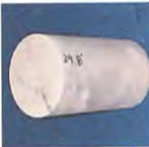
Louisville Tunnel Project 1831-10-5629 South Bound Boring 30 (Run 151 Box 101) 1,430.0' (Unconfined)
