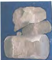
Louisville Tunnel Project 1831-10-5629 South Bound Boring 33 (Run 157 Box 105) 1,489.8' (Unconfined)
