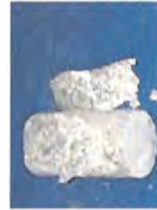
Louisville Tunnel Project 1831-10-5629 South Bound Boring 2 (Run 46 Box 33) 416.7' (Unconfined)
