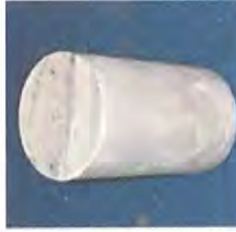
Louisville Tunnel Project 1831-10-5629 South Bound Boring 18 (Run 125 Box 85) 1,185.2' (Unconfined)
