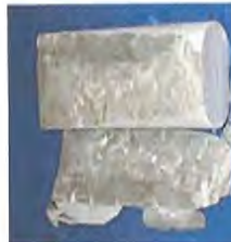
Louisville Tunnel Project 1831-10-5629 South Bound Boring 27 (Run 145 Box 97) 1,371.0' (Unconfined)
