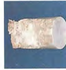
Louisville Tunnel Project 1831-10-5629 South Bound Boring 10 (Run 94 Box 65) 885.2' (Unconfined)
