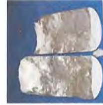
Louisville Tunnel Project 1831-10-5629 South Bound Boring 4 (Run 58 Box 41) 533.7' (Unconfined)
