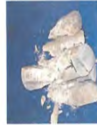
Louisville Tunnel Project 1831-10-5629 South Bound Boring 6 (Run 70 Box 49) 652.4' (Unconfined)
