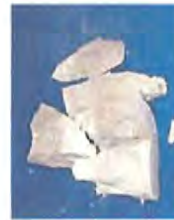
Louisville Tunnel Project 1831-10-5629 South Bound Boring 1 (Run 40 Box 29) 354.6' (Unconfined)
