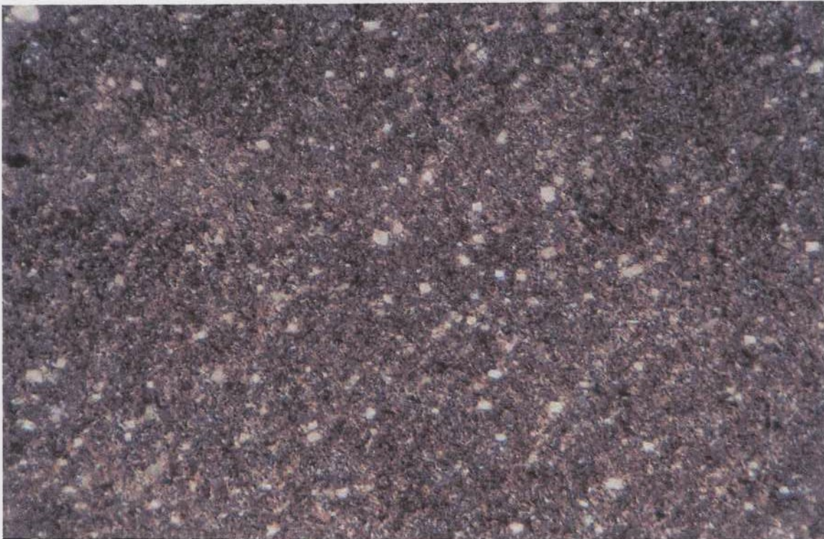
B-7-4 @ 87.1-87.3. Matrix of fine-grained calcite mud (brown, speckled) hosts secondary dolomite crystals (bright, diamond-shaped), and encloses or isolates them from contact with each other. Field of view 2.4 mm at 40X, taken under crossed polars.
