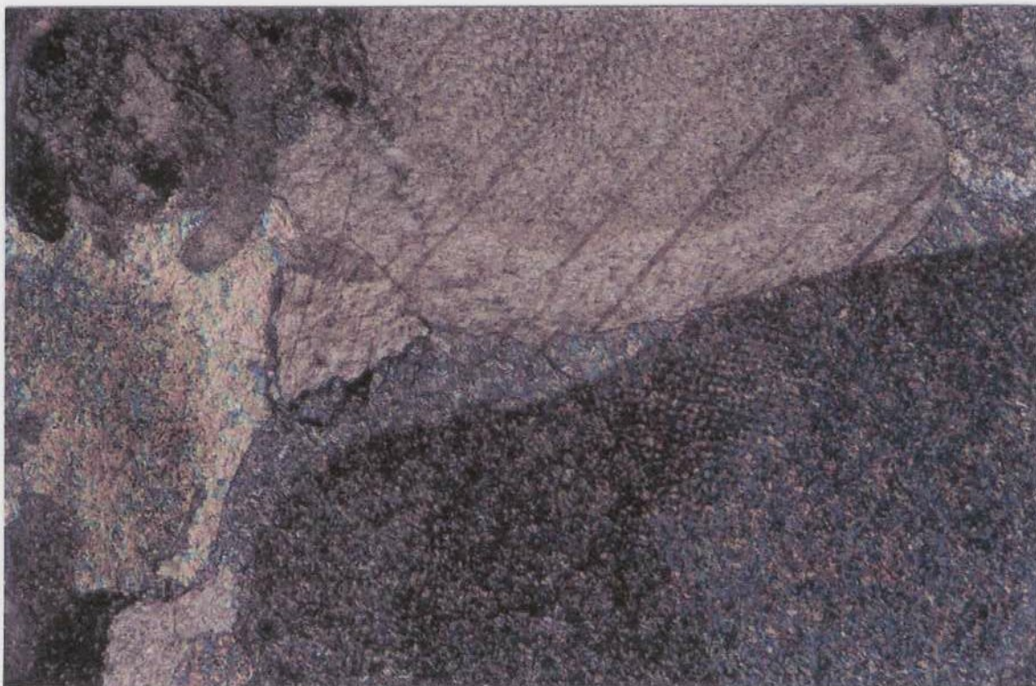
B-14-3 @ 87.1-87.6. Large fossil fragments interlock along long, straight boundaries and angular boundaries. Field of view 2.4 mm at 40X, taken under crossed polars.
