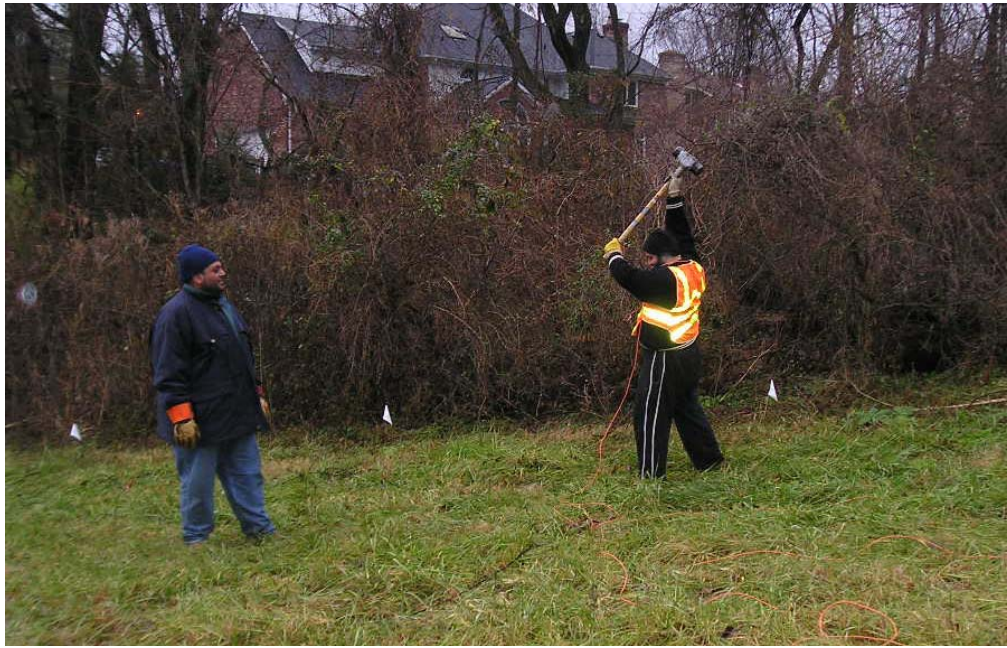
Figure 9: A 20 pound sledge hammer was used as an acoustic source.
