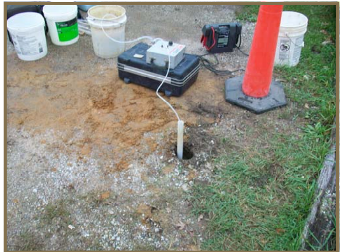
Low-flow sampling of temporary monitoring wells.
