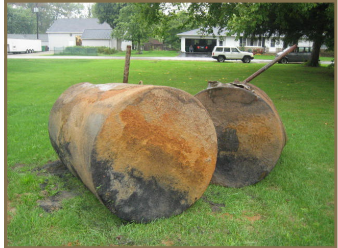
Two 550-gallon underground storage tanks
