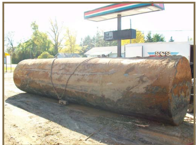
Gasoline UST that was removed awaiting a trip to the landfill.
