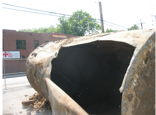
UST after removal with visible holes
