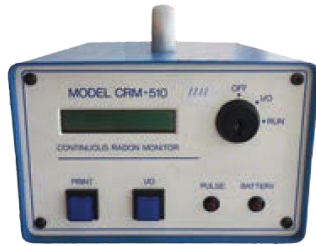
Continuous radon monitor (CRM)
