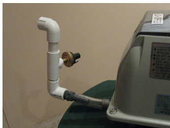
Figure A1: Air supply pipe connection to air pump with sensor attached.
