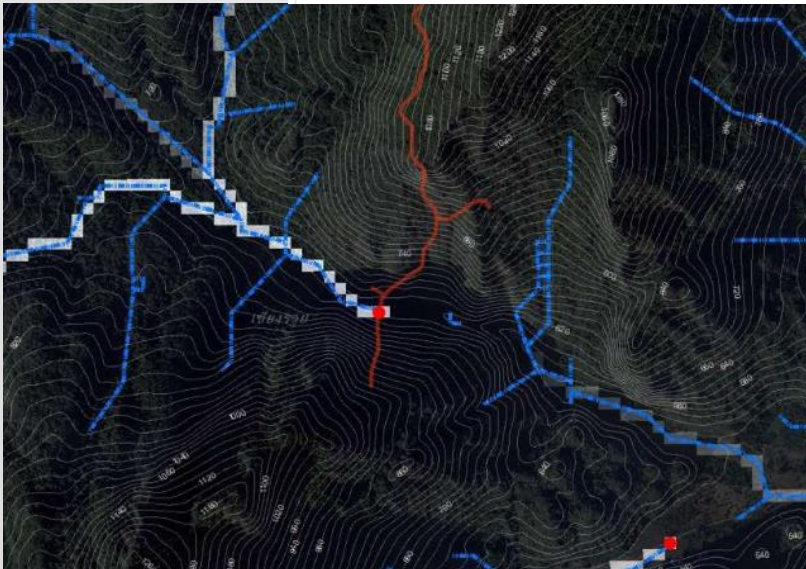
A 3D map showing the extent and direction of water flow on the hill in relation to the cave below helped to pinpoint the placement of dams and pipes that greatly reduced the rise of water.
