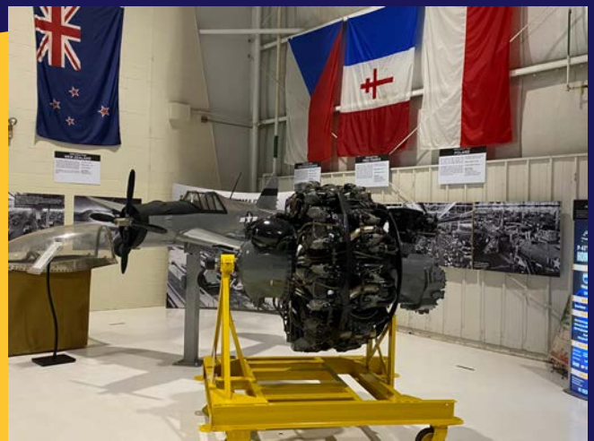
The Thunderbolt was effective as a short- to medium-range escort fighter in high-altitude air-to-air combat and ground attack in both the European and Pacific theaters. The P-47 was designed around the powerful Pratt & Whitney R-2800 Double Wasp 18-cylinder radial engine, which also powered two U.S. Navy/U.S. Marine Corps fighters, the Grumman F-6F Hellcat and the Vought F-4U Corsair. An advanced turbosupercharger system ensured the aircraft's eventual dominance at high altitudes, while also influencing its size and design.
