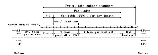
MULTI-LANE DIVIDED WITH SINGLE OR TANDEM OVERHEAD STRUCTURES AND SHOULDER PIER TO E.P. > 16'-0
