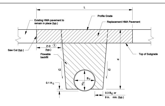
L = Longitudinal pay limits of pavement removal and pavement replacement (ft)
