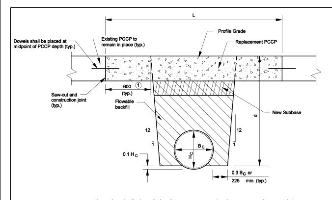
L = Longitudinal pay limits of pavement removal and pavement replacement (m)
