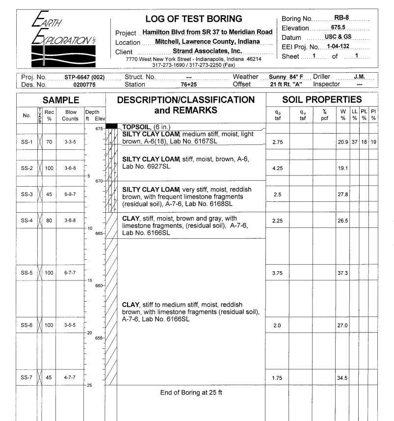
Drilling Method 31/4" I.D. HSA Remarks Backfilled with auger cuttings and NW NW NW To Water bentonite chip plug near surface. 21 To Cave-in 21 The stratification lines represent the approximate boundary between soil/rock types and the transition may be gradual.
