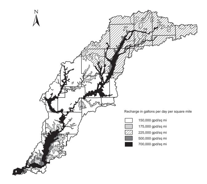
Figure 13a. Estimated recharge rates of unconsolidated aquifer systems
