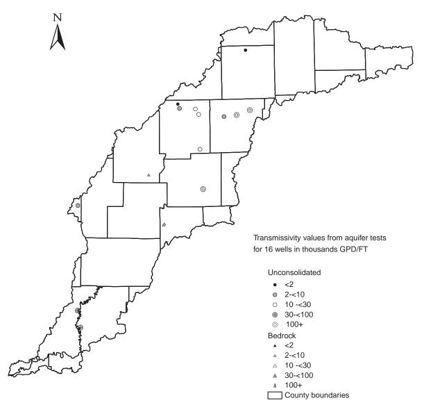
Figure 12. Transmissivity estimates from aquifer tests
