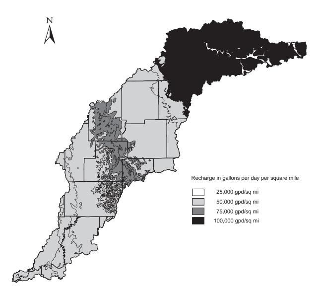
Figure 13b. Estimated recharge rates of bedrock aquifer systems
