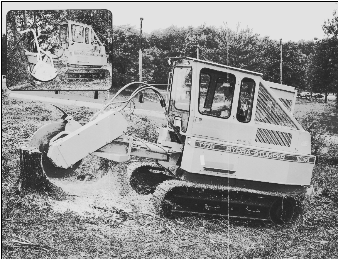
Exhibit 304a: Example of Equipment Used for Stump Removal (Source: C&S Equipment Sales, Inc.)
