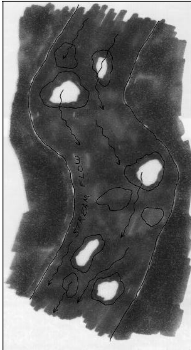
Exhibit 1202c: Boulder placement (Source: Forest Service Habitat Improvement Handbook)
