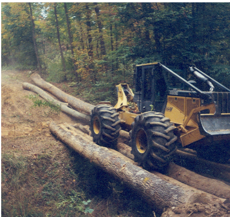
A skidder crosses a log bridge.
