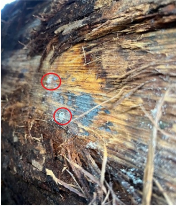
Photo 9 – Recent possible powderpost beetle activity in White Oak ( Quercus alba ) log. Damaging powderpost beetle species in the area normally consist of either anobiid beetles, bostrichid beetles, or lyctid beetles. Powderpost beetles can be distinguished by their fine sawdust piles near the emergence holes (note circled areas in photo)
