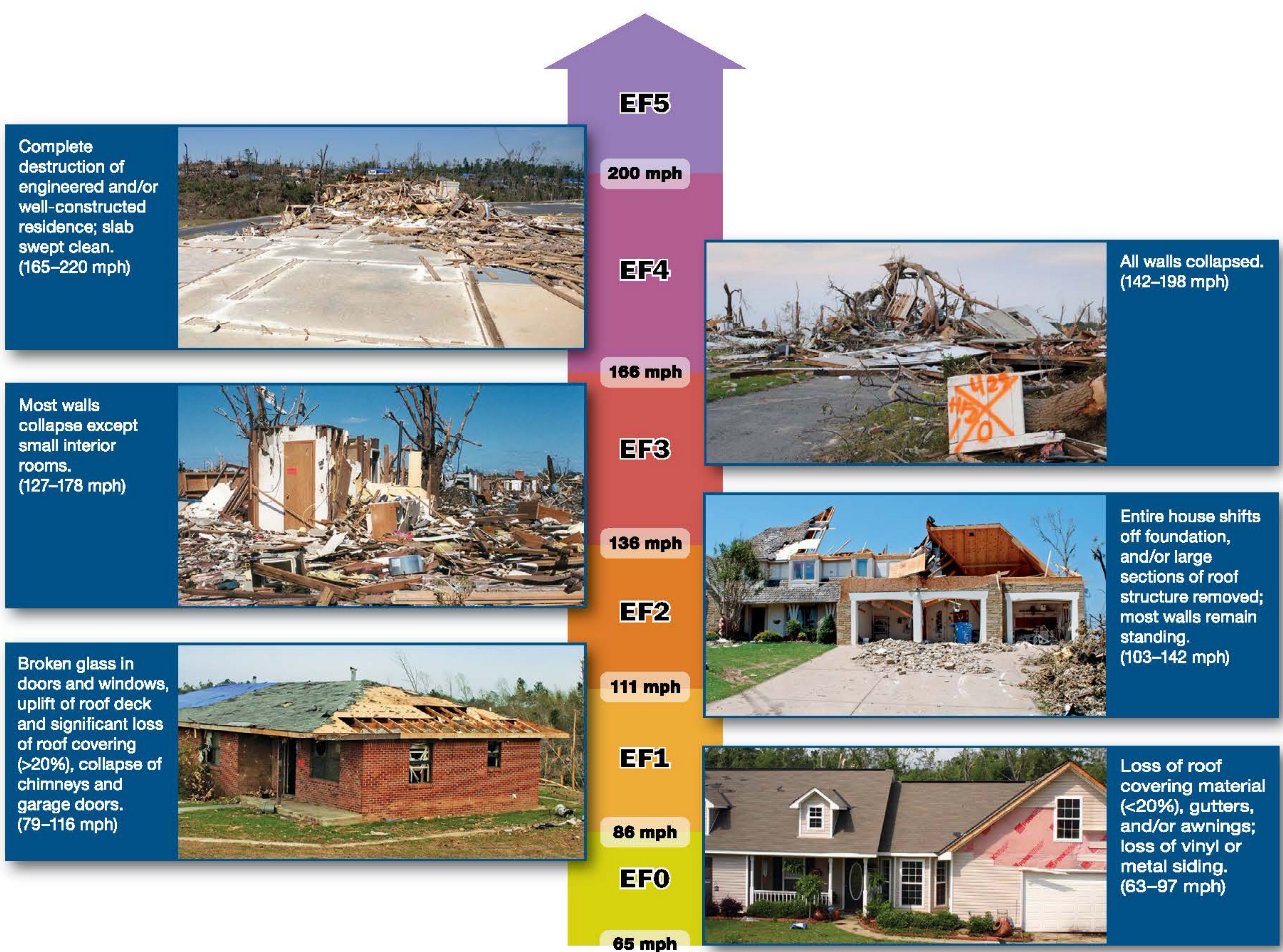
Figure A2-1. Typical tornado damage descriptions to one- and two-family dwellings and their corresponding intensity according to the EF Scale (wind speeds are estimated 3-second-gust wind speeds)
