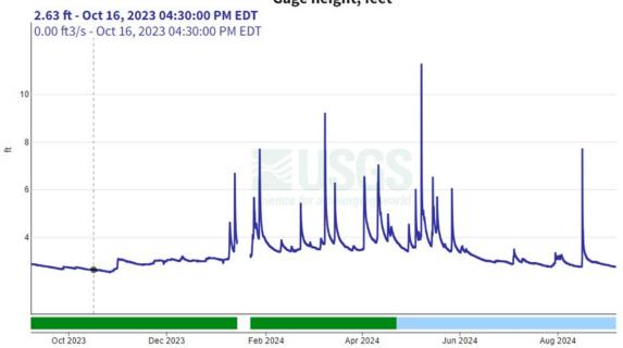
Continuous monitoring of the volume of water that flows into the lake, specifically during storm events, is crucial and allows for year-to-year data comparison. It also enables partners to sample for pollutants during periods of high flow. This can help identify specific strategies that we should take to reduce run-off of sediment and 'nutrients' from fertilizers, farm chemicals, animal waste and septic waste.
