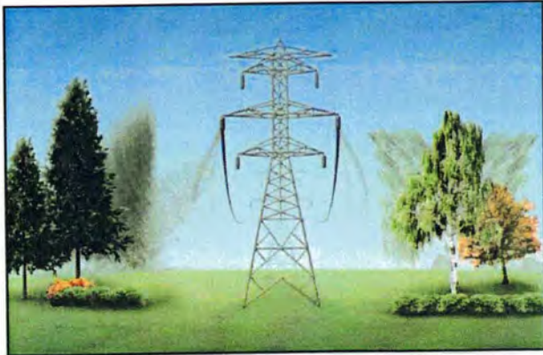
Fall distance of trees needs to be considered in placement of new plantings.
