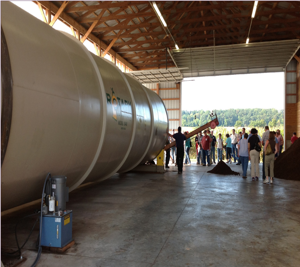
Figure 6-13. Rotating drum for carcass composting
