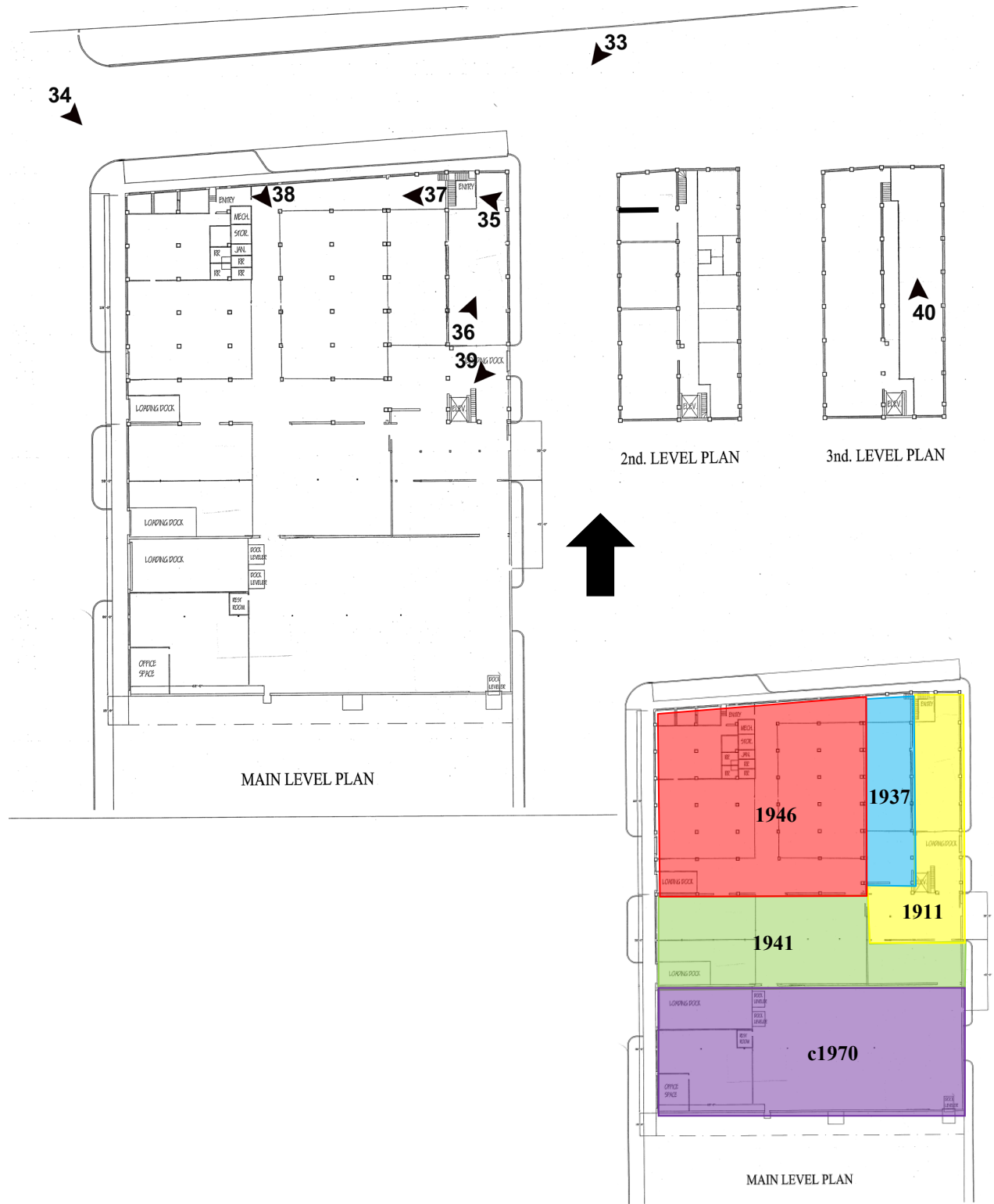
Figure 25. Stutz II photo maps. Bottom right is a diagrammatic key to building and additions dates. Base maps provided by owner.
